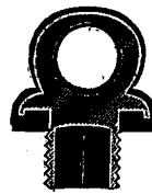
The Patent Rubber Covered Screw Stopper, No. 107940, in section.
